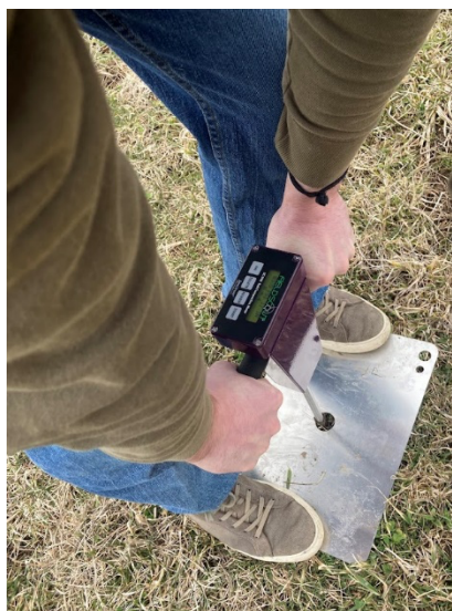
Photo: Obtaining a soil penetrometer reading from an undisturbed area adjacent to the bale grazed site in spring 2024.
