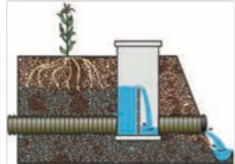
Figure 3. The outlet is raised after planting to potentially store water for crops.
