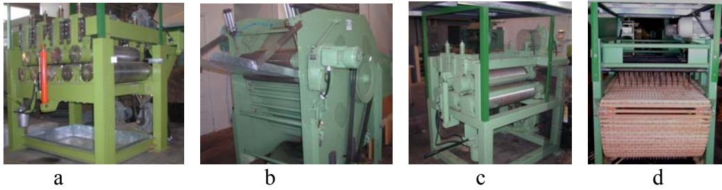
Figure 2. Four modules comprising the USDA Flax Fiber Pilot Plant. a. Nine-roller crushing calender. b. Scutching wheel that aggressively cleans and shortens fibers. c. Five-roller calender with grooved surfaces to further clean fibers. d. Top shaker with arching prongs and pinned apron to remove shive and partially align fibers. Adapted from Akin et al., 2004a
